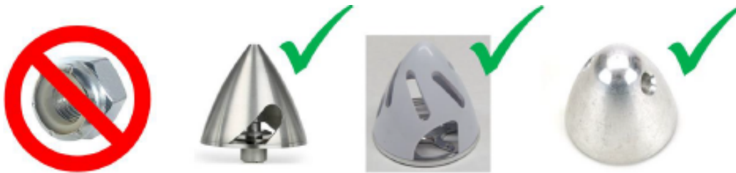
Figure 3.2: Permitted and prohibited devices to secure the propeller
